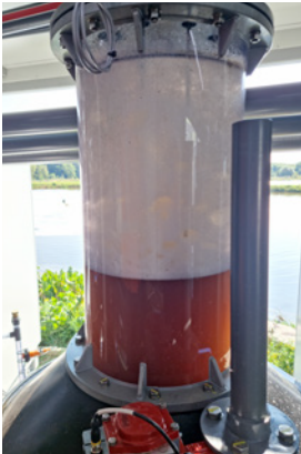
Figure 3: Photo taken during the second fractionation step in a full-scale plant. The dry foam can be seen being removed by vacuum.
